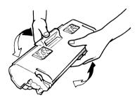
6 Slide the pins located on both sides of the Imaging Cartridge into the grooves of the printer as shown and gently push the Imaging Cartridge securely into place.
